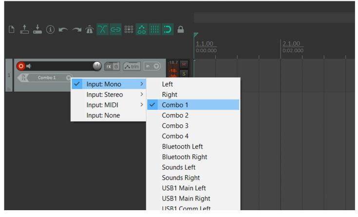
**NOTE:** The multitrack output configuration is always the same, regardless of how you have your mixer set up. For example, if you have combo input 2 assigned to fader 6 on your mixer, it will still appear on input 4 in your DAW. Also, if you do not have an audio input allocated to a fader on the mixer, it will not pass through to the multitrack output, so it's a good idea you have your mixer configured
