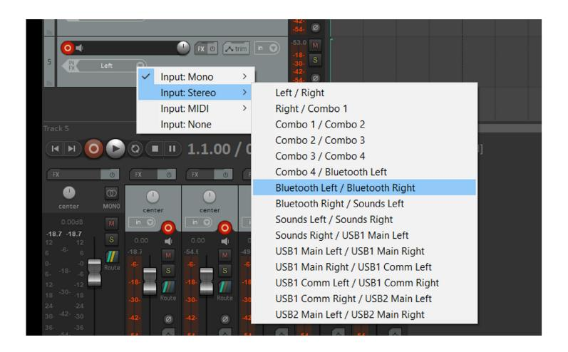
Create a new track by double clicking on the area underneath the existing tracks (you can scroll the display to do this if necessary) and click the 'record' button.
